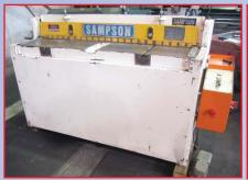
**SAMPSON** 4'X 14 GAUGE HYDRAULIC SHEAR, MODEL LB-414H
